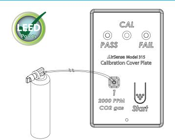
Your sensor comes factory-calibrated and does not need to be calibrated upon initial installation. Calibration kits are available and include all the necessary elements, including a 17 liter cylinder of 2000 PPM calibration gas (enough gas to calibrate 15-20 units). Recommended calibration interval is 5 years.
