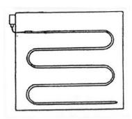
Fig A. Proper Installation of Capillary Element
