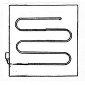
Fig C. Control Case and Capillary Element Installation which is NOT RECOMMENDED
