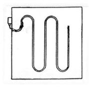
Fig B. Improper Installation of Capillary Element
